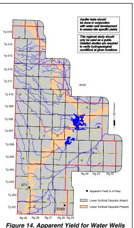
Figure 14. Apparent Yield for Water Wells Completed into Lower Surficial Deposits
