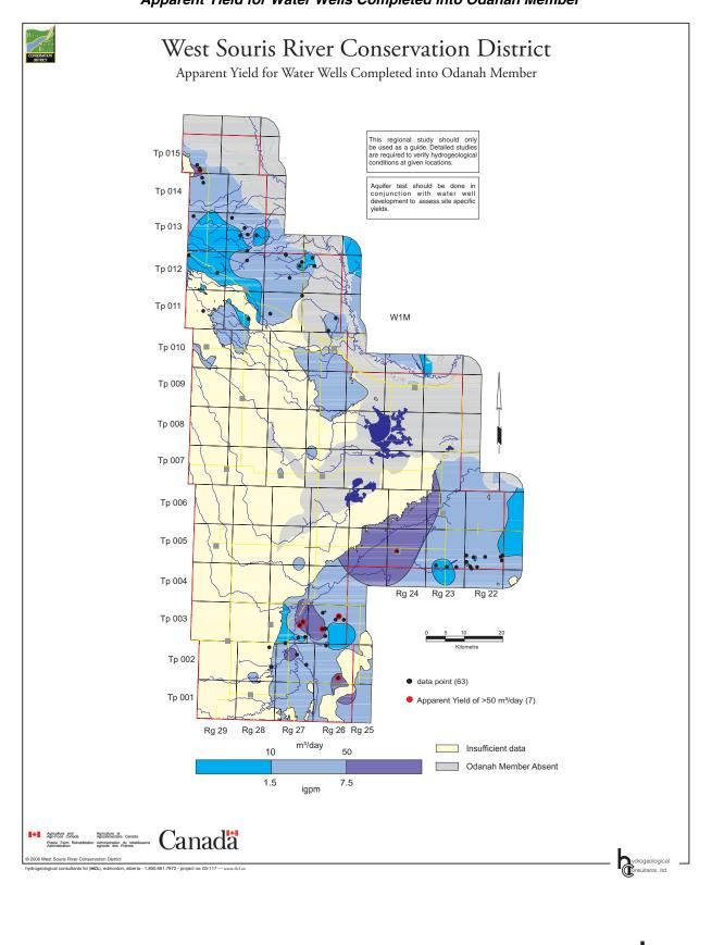
Apparent Yield for Water Wells Completed into Odanah Member
