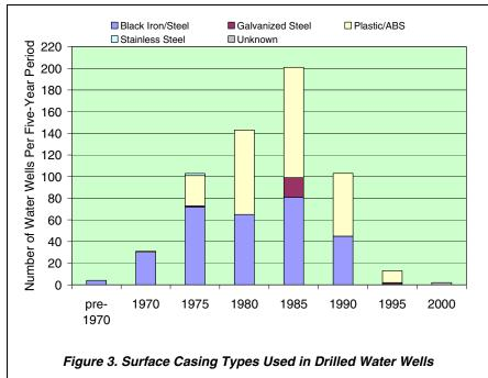
Galvanized steel surface casing in drilled water wells was first used in the Study Area in October 1977 and was used in eight percent of the drilled water wells from 1995 to 1999.
