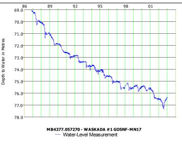
Figure 22. Hydrograph – Waskada #1 Monitoring Water Well
