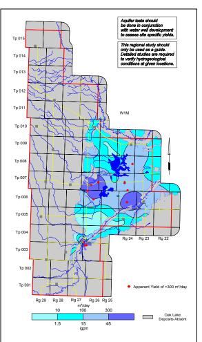
Figure 11. Apparent Yield for Water Wells Completed into Oak Lake Deposits
